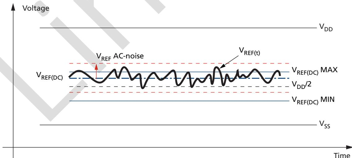
The voltage levels for setup and hold time measurements are dependent on  $V_{REF}$ .  $V_{REF}$  is understood as  $V_{REF(DC)}$ , as defined in the above figure. This clarifies that DC-variations of  $V_{REF}$  affect the absolute
